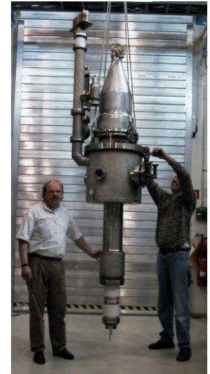
Gyrotron, 2.2 MW peak at 170 GHz
